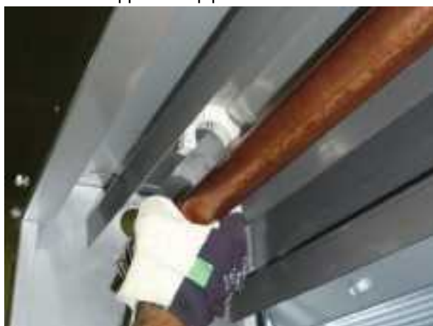
Release copper collector from plastic holders
