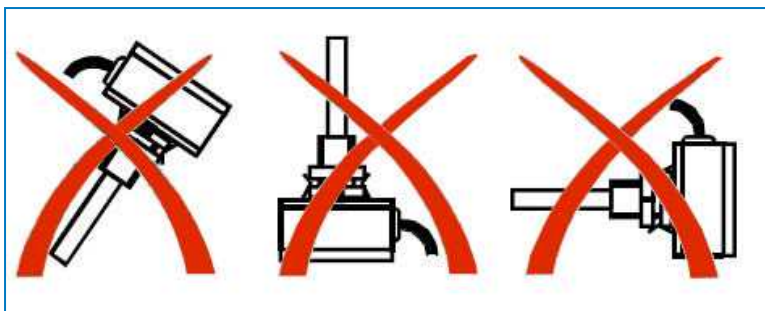
Not permitted positions for mounting VFD sensor
